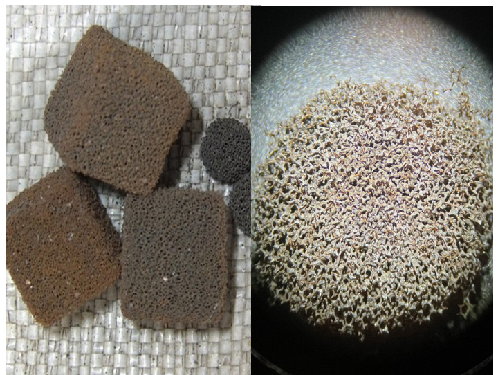
Foam-type carrier: virgin material (left) and abraded material (right).
