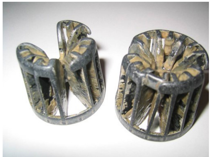
Abrasion of carrier media in operation.
