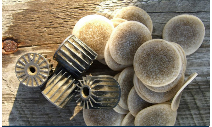
For comparison: clogged carrier (left) and unclogged carrier (right).
